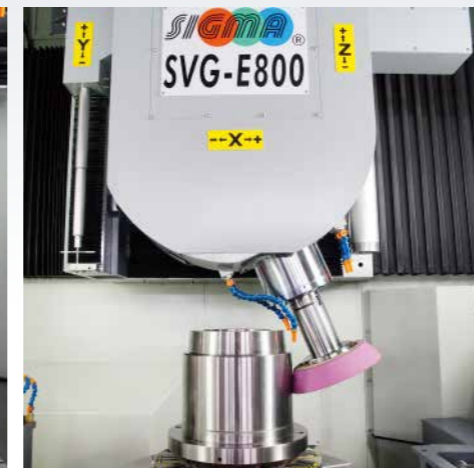
OD cylindrical grinding (grinding spindle at 22.5 degrees)
