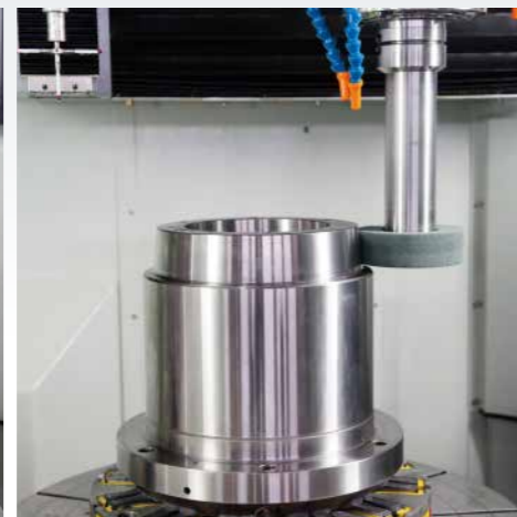
2-axes simultaneous OD cylindrical grinding (slop 5 degrees)
